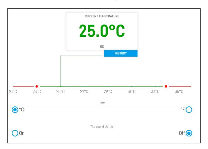
When the temperature exceeds the limit (default is 23°C and 27°C) Thermo view will send a notification to your devices letting you know. If the sound alarm is turned on it will start audible alarm as well.
