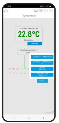
In the device menu, press the "SETTINGS" button, and then select "TEMPERATURE CALIBRATION" from the drop-down menu.
