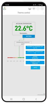
After the calibration process, the Thermo control device will indicate the corrected temperature in the menu, and when you press the "SETTINGS" button again, information about the value of the measurement difference after calibration will additionally appear. A value of -0.2 means that the temperature value you entered is 0.2 units lower than the value measured before calibration.
